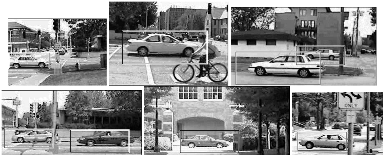
Fig. 14. Examples of test images on which our multi-scale detection system achieved perfect detection results. Results shown are with the neighborhood suppression algorithm (see Section II-D) at the point of highest F-measure from Table IV, i.e. using an activation threshold of 0.95. The windows are drawn by a separate evaluator program at the exact locations and scales output by the detector.
