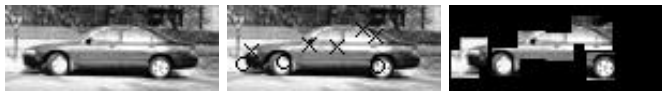
Fig. 1. Left: A sample object image used in vocabulary construction. Center: Interest points detected by the Förstner operator. Crosses denote intersection points; circles denote centers of circular patterns. Right: Patches extracted around the interest points.
